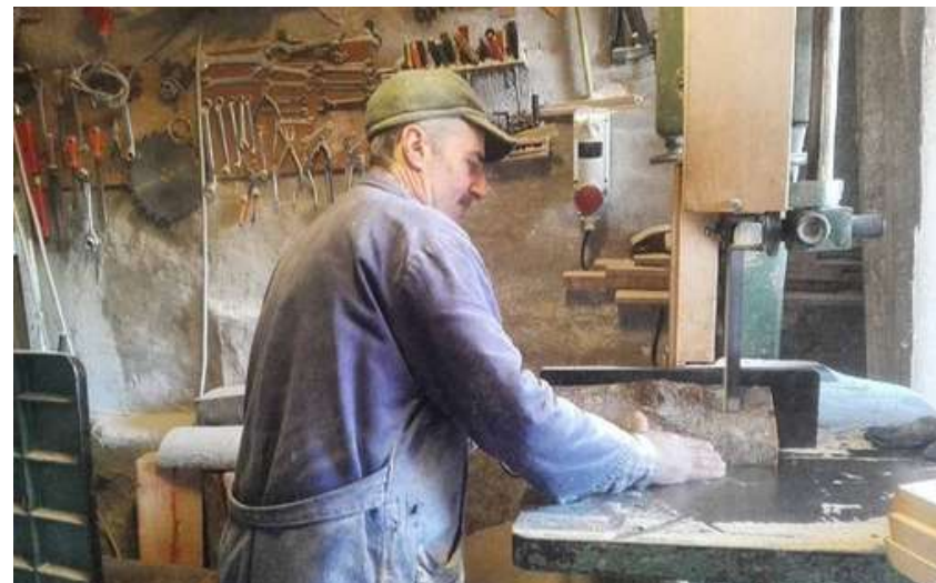
There are 20 steps to make a chitarra and it takes time, patience, and skills. Wood is cut, the pieces are carved, shaped, drilled, and polished.
