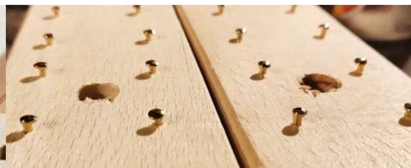
Little nails are inserted to hold the steel strings (hence the name chitarra , which means "guitar"). 45-50 metres of wire are strung on the frame.
